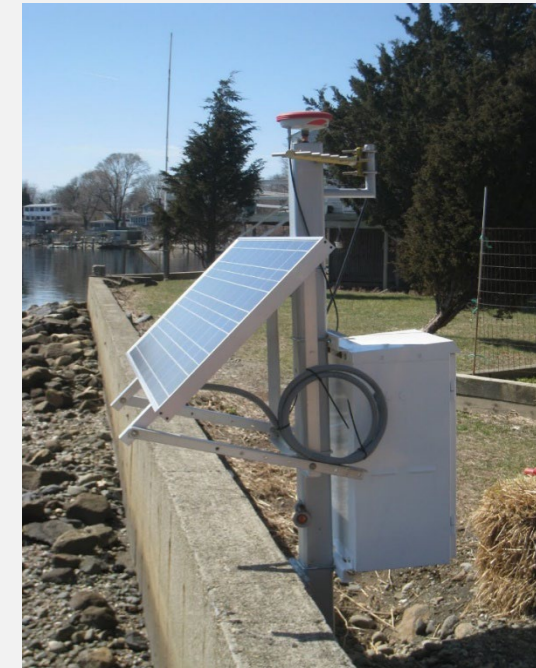
dGPS station – GPS, spread-spectrum radio, solar engine
